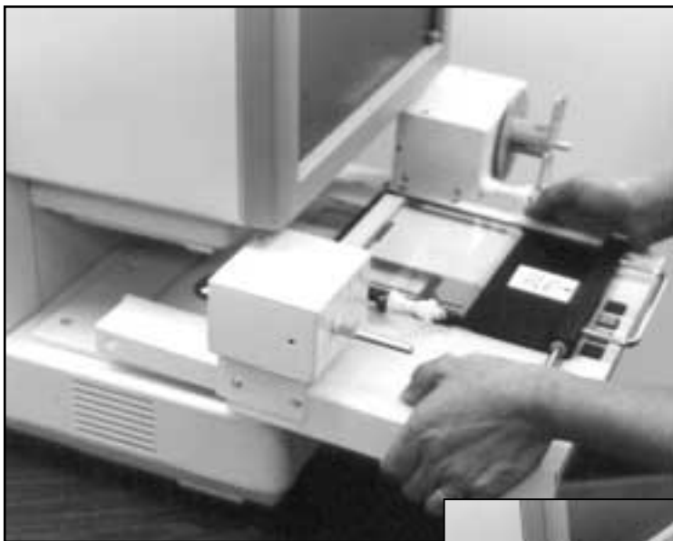
A. Center the Combo Carrier on the hook at the rear of the carrier stage (see photos on previous page).
