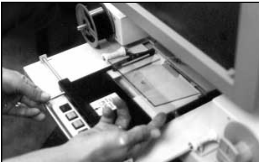
TO THREAD FILM: Pull handle to open top glass, then load film on the left spindle.
