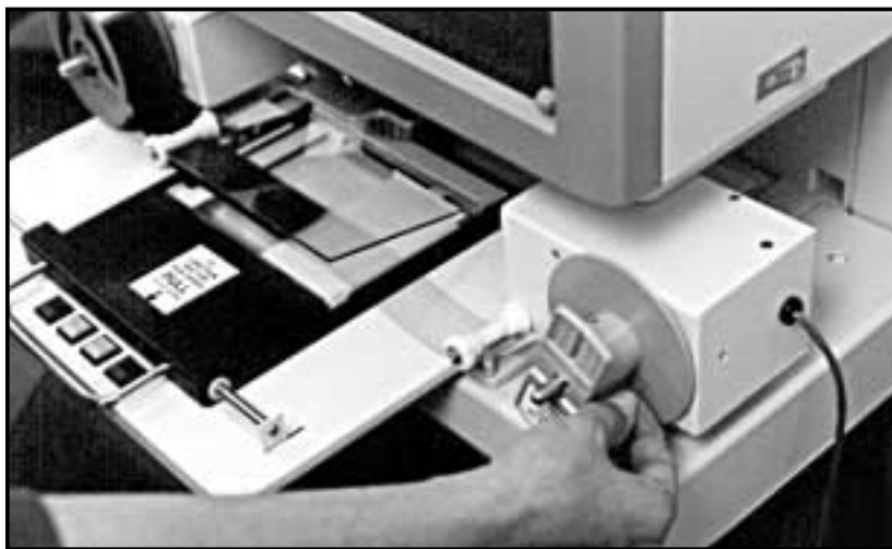
Feed film from over the top of the reel, under first white guide roller, between glass flats, under second guide roller and into the take-up reel slot.
